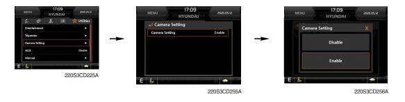
· In the operation screen, rear camera screen shows up when ESC/CAM switch is pushed.
