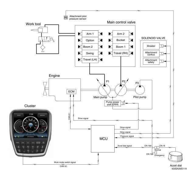
• The system is used to control the pump delivery flow according to set of the work tool on the cluster by the attachment flow EPPR valve.
