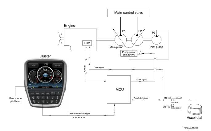
1) High idle rpm, auto idle rpm and EPPR pressure can be adjusted and memorized in the U-mode.
