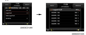
The logged faults of the MCU can be checked by this menu.
