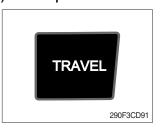
① This switch is used to select the travel speed alternatively.
